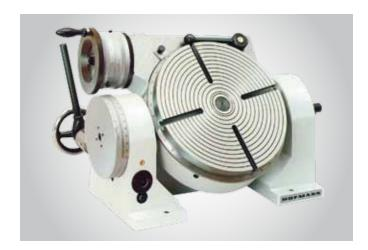
Manual tilting rotary table HPRS available with table plate diameters of 250, 320 and 400 mm, tilting range from 0° to 90°. There are the following designs:
