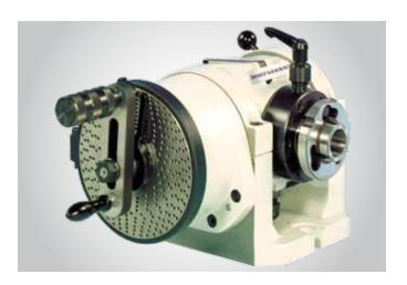
Semi-universal dividing head HTH with manual rotary and tilting axis, available with center heights 100, 125, 160 and 200 mm. The rotary axis can be tilted from 0° to 90°.
